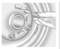
Reinstall the wheel nuts with the rounded end of the nuts toward the wheel. Tighten each nut clockwise by hand until the wheel is held against the hub.
